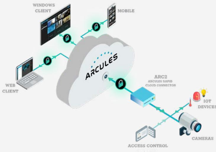
**\*\*ARC<sup>2</sup> appliance supports up to 30 channels. An ARC<sup>2</sup> appliance is required for each site.**
